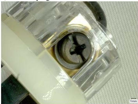
Figure 30. Optical images of the plug used to connect the standard receptacle to the GFCI receptacle in Circuit 1. The prongs and screws are blackened relative to those on a new, as-received, unexposed plug.
