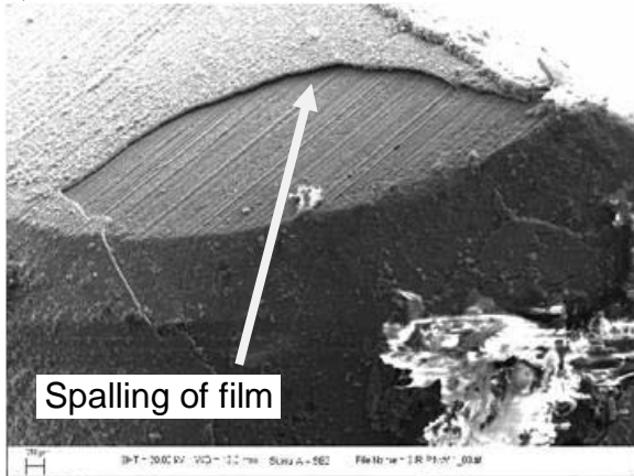
Figure 54. SEM images of the surface of the neutral wire from the receptacle in Circuit 3. The connection was a push-in connection. (B) shows the contact point, which is brighter due to the presence of Cu without S. The end of the wire is shown in the lower images at two magnifications. Note the spalling of the corrosion product film. It is believed that the spalling occurred during the test, but is it possible that it occurred after exposure and prior to analysis.
