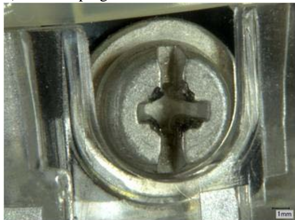
Figure 30. Optical images of the plug used to connect the standard receptacle to the GFCI receptacle in Circuit 1. The prongs and screws are blackened relative to those on a new, as-received, unexposed plug.
