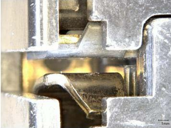
Figure 29. Optical images of the contacts in the standard circuit breaker in Circuit 1.
