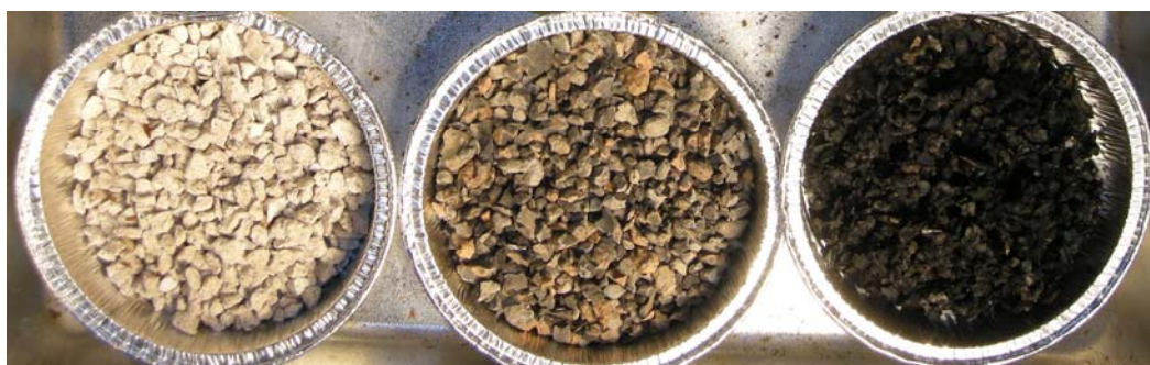
Figure 18 Stage 1 Media, Upper Layer Dried at 103C (Day 246). Left to right: clinoptilolite, expanded clay, granular rubber.
